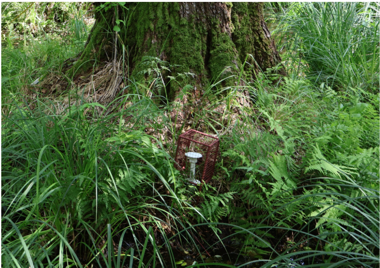
TOMS-T humidity logger with protective cage at NERVE4 plot
